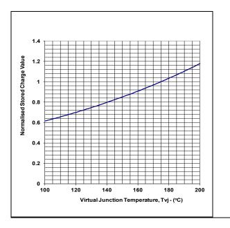
Fig 5 Stored Charge against Junction Temperature
