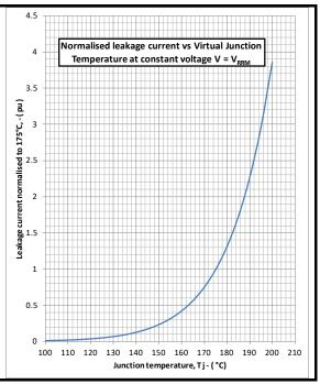
Fig. 1 Leakage current vs junction temperature
